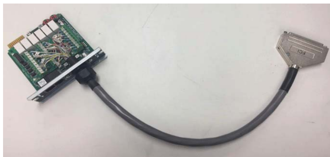
FIG. 1. Photo of relay card with terminal block connections wired to 37-pin D-sub connector.
